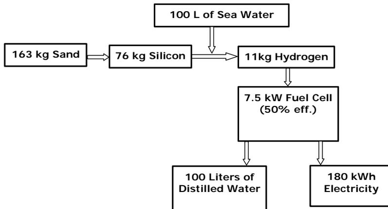
**Figure 5: Production of drinking water as a byproduct of power generation using sand**
